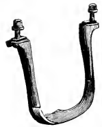
FIG. 107.—Onion harvesting attachment for wheel hoe.
